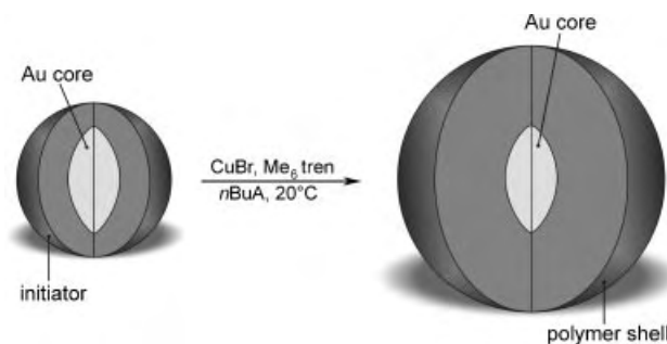
Figure 1. Generation of a polymer shell around the Au-NPs; n BuA = n -butylacrylate.
